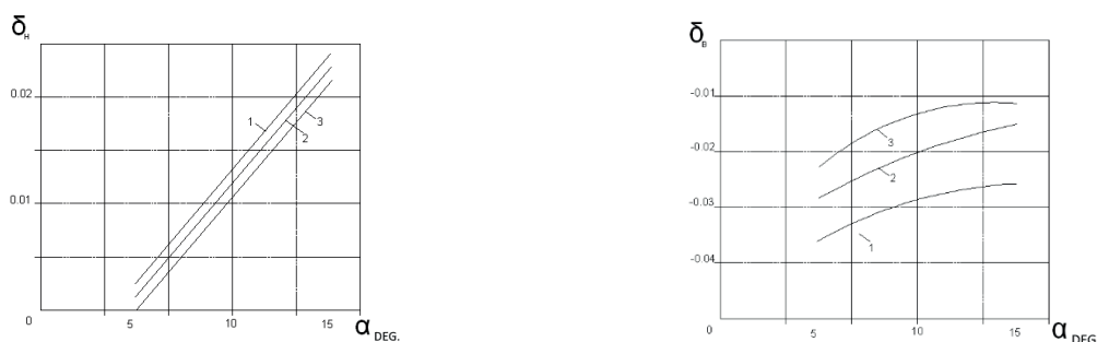
Figure 1 The dependence of certain parameters of the on-board slip coefficients of a 5VS-15M mechanical vehicle on the angle of rotation of the wheels Note: 1 - at a = 1.25 ; 2 - at a = 1.47 ; 3 - at a = 1.75
