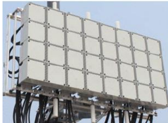
Fig. 7: Masive MIMO antenna
