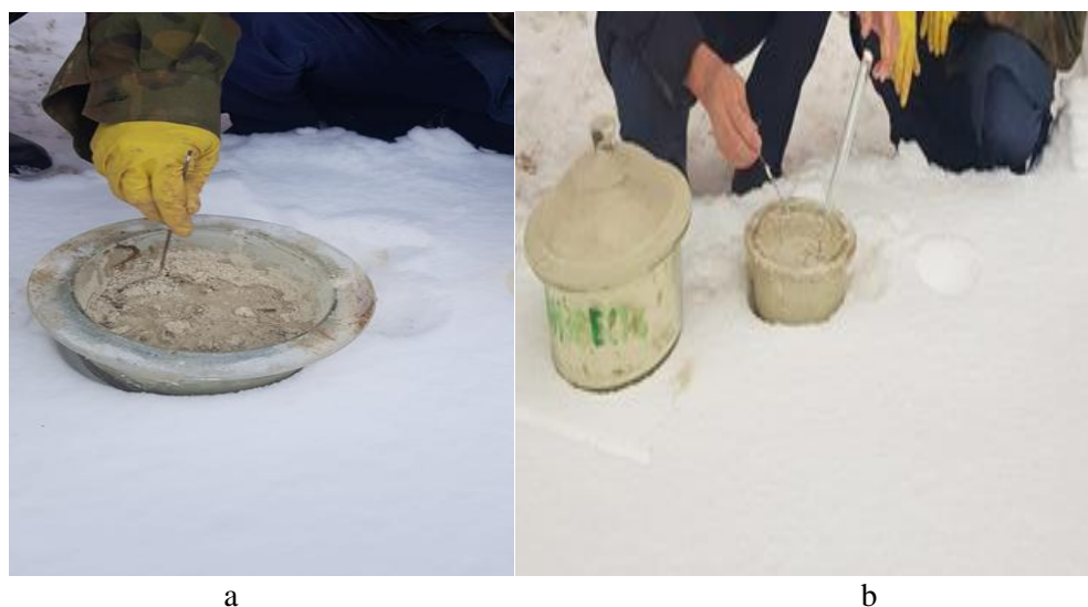
Figure 3. Fragments of preparation of a laboratory sample of seasonally frozen soil at ambient temperature t = -20^{\circ}\text{C} : a – laboratory sample of seasonally frozen soil; b – preparation of samples for experiments
