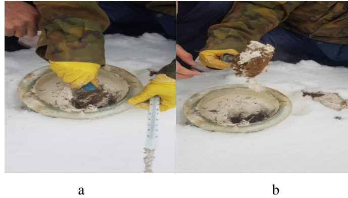
Figure 6. Fragments of a thawed sample of seasonally frozen soil when using a chemical reagent based on quicklime: a – the process of checking the thawed laboratory seasonally frozen soil; b – the appearance of a completely thawed sample of frozen soil
