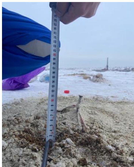
Figure 7. Measuring the thawed depth first day
