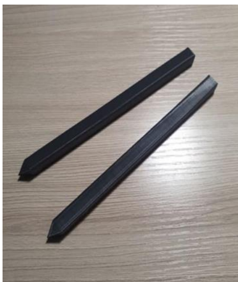
Figure 2. The model piles made of plastic
