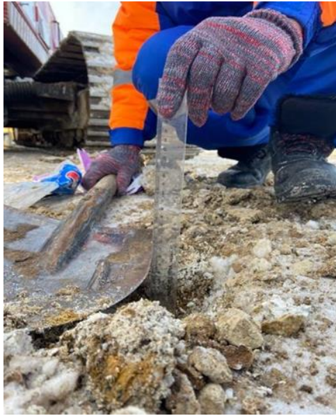
Figure 8. Measuring the thawed depth third day
