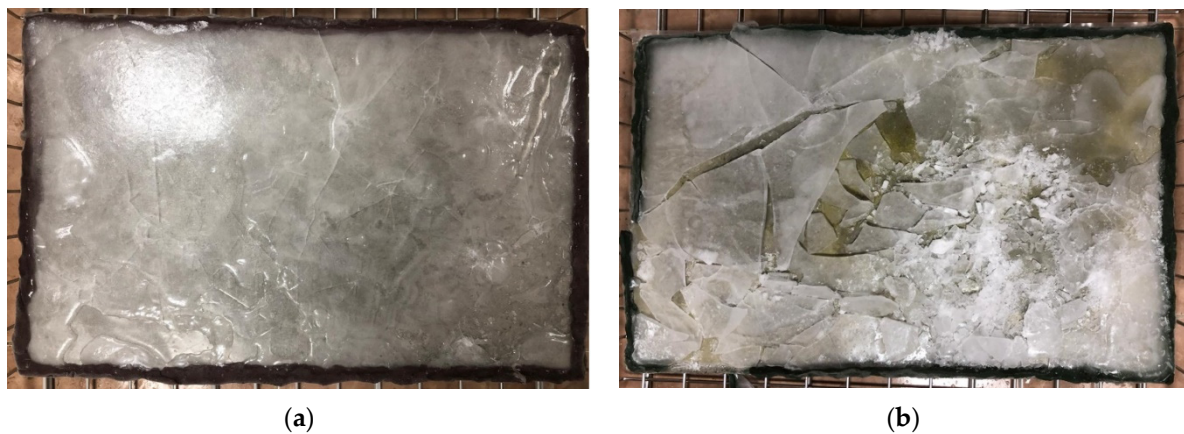
Figure 5. Specimens after vibration test. (a) Not coated, (b) Coated.
