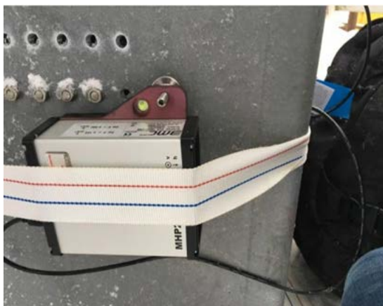
Fig. 11 Location of the accelerometers (position of sensor at level 36 m)
