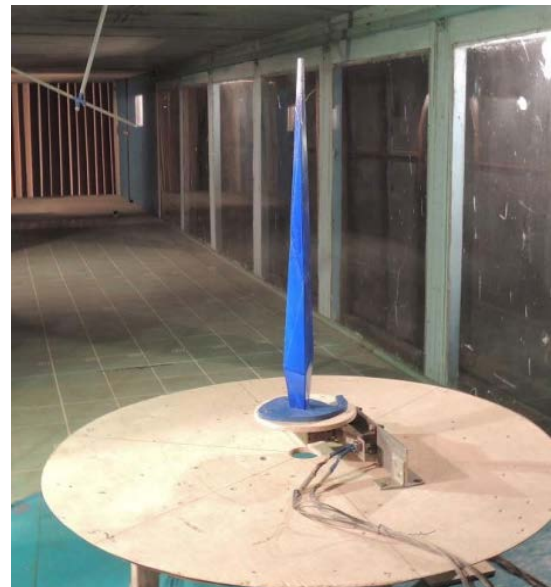
Fig. 3 General view of the building model in a wind tunnel
