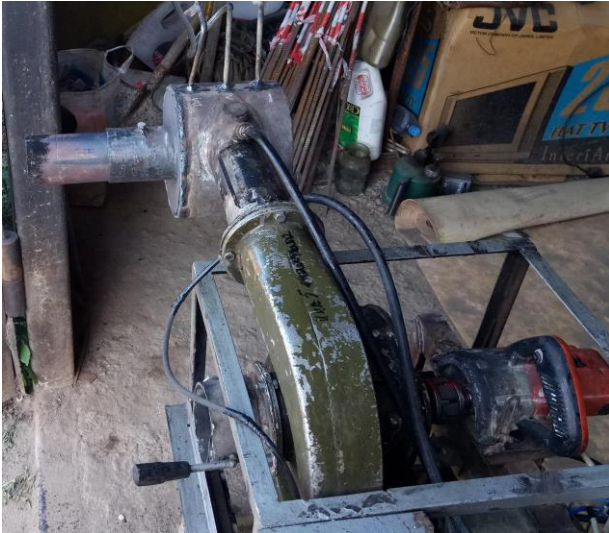
Fig. 3. Experimental burner with a mobile discharge nozzle.
