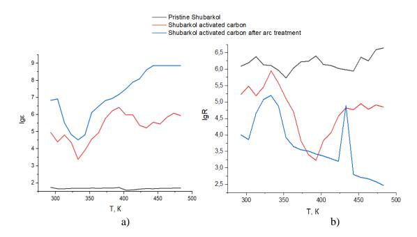
Figure 4 Dependence of dielectric constant (a) and electrical resistance (b) on temperature at a frequency of 1 kHz
