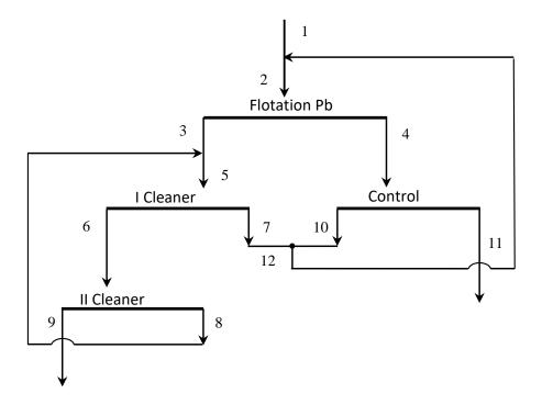
Figure 2 - Lead Flotation Cycle
