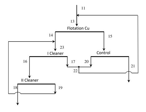
Figure 3 – Copper flotation cycle
