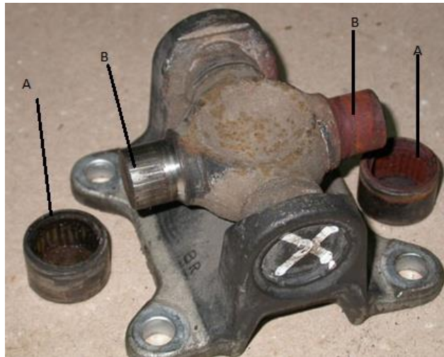
Figure 3. The appearance of worn parts ("false brining") of the bearing assembly of the crosspiece a) – bearing cage; b) – the axle of the crosspiece
