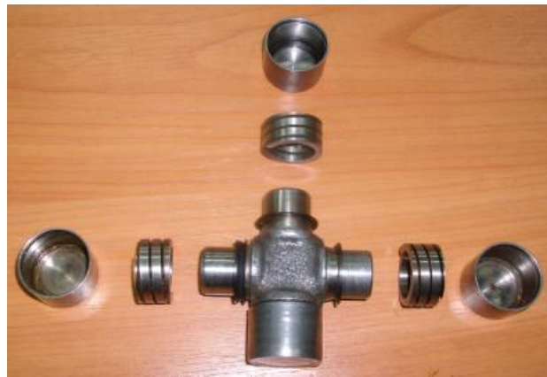
Figure 4. The upgraded crosspiece of the VAZ "Niva" car
