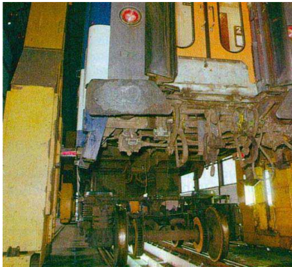
Figure 2 – Changing bogies in a passenger coach
