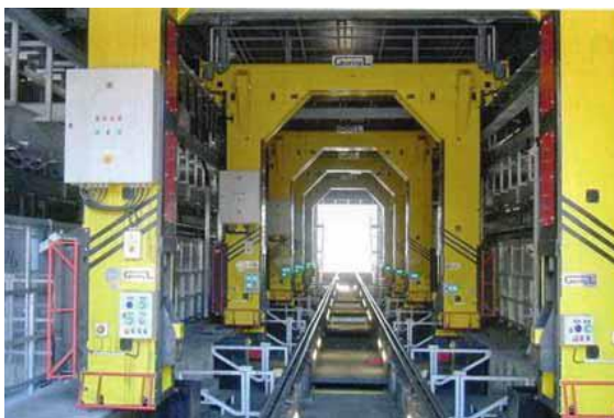
Figure 1 – Wagon axle interchanger
