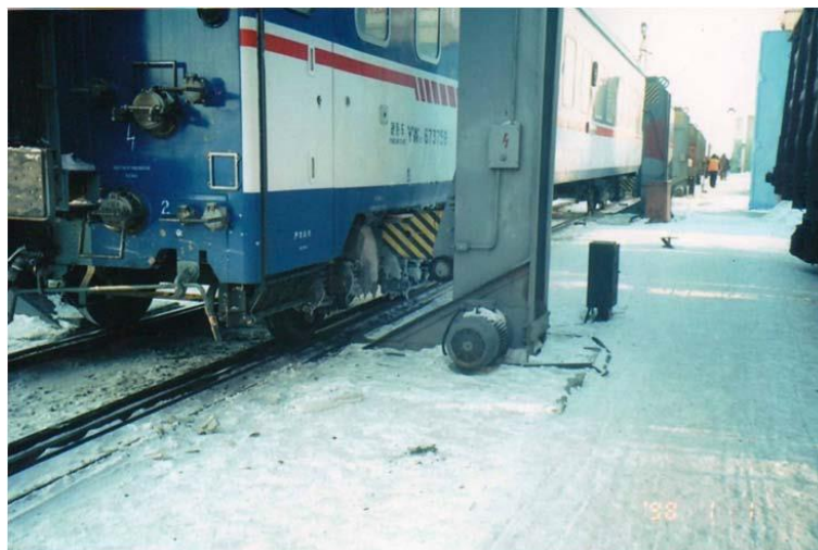
Figure 3 – Changing bogies in a passenger coach
