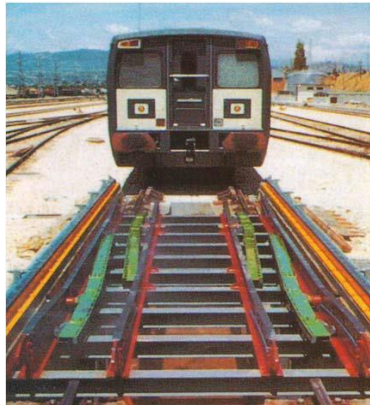
Figure 5 – Pattern of TalgoRD rail track changing system
